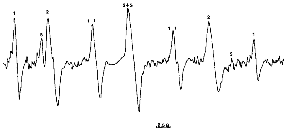
Fig. 1. The ESR spectrum observed during irradiation of nitrogen-saturated aqueous solution of DAA ( 10^{-3} M) in the presence of NtB ( 1 \text{ mg ml}^{-1} ).
